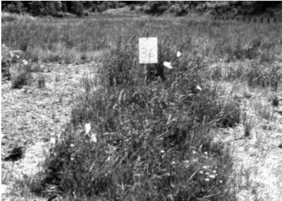
Figure 5. Vegetation response to surface blended fly ash (approx 50% ash blended to 6 inches) at Pine Branch refuse pile experimental plots (see Table 4) two years after application. The bare plot to the left is an untreated control plot.
