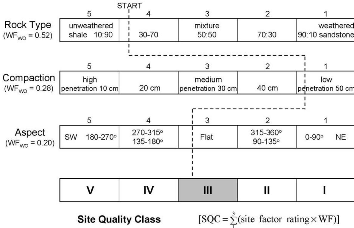
**Figure 1.** Site factor gradients used to determine overall mined site quality class (SQC). The field mapping criteria, rock type, level of compaction and aspect, are scored from 1 to 5 and the score is adjusted by multiplying by their respective weighting factors (WF). SQC is determined by summing the adjusted scores (Burger et al. 2002). The word “Start” shows an example culminating in a SQC III.
