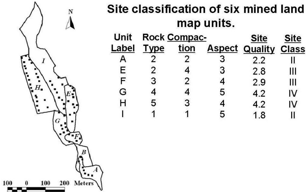
**Figure 2. Soil/site quality classification and mapping of the Rapoca reclamation site in southwestern Virginia. The data points on the map indicate locations of selected white oaks that were used to test the classification criteria. Values are based on the site quality class scheme in Figure 1.**
