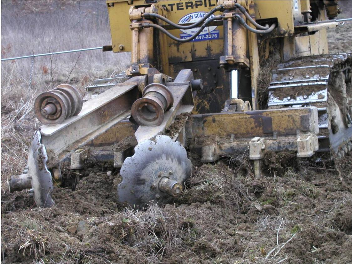
**Photo 1. An advanced ripping tool used to prepare the biomass research sites by Union Concrete Products of Maxwellton, West Virginia, under the direction of J. K. Rose.**
