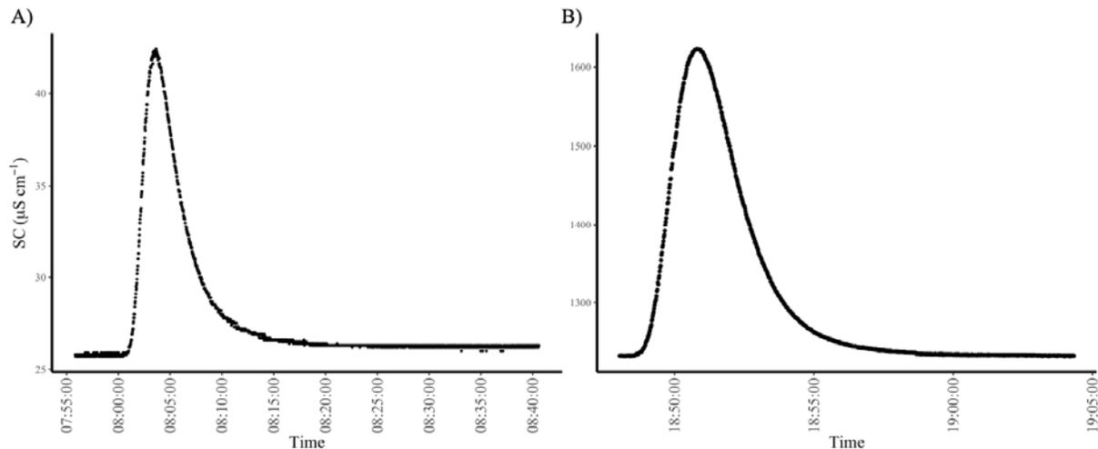
**Figure 3:** Recorded SC wave created from salt slug additions to a reference stream (A) and a salinized stream (B). The area under the curve is used to calculate stream flow at a given point in time and water level.
